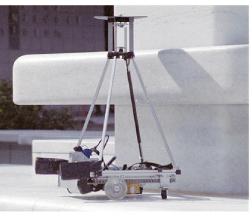
The VolksBot is a modular lightweight robot and can be easily adapted for specific needs, in this case RoboCup.
